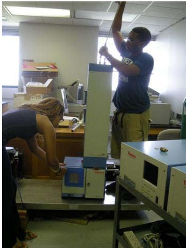
Figure 2. Students Avian Lain and LaMarr Hill working on the installation of TEOM 1405.
