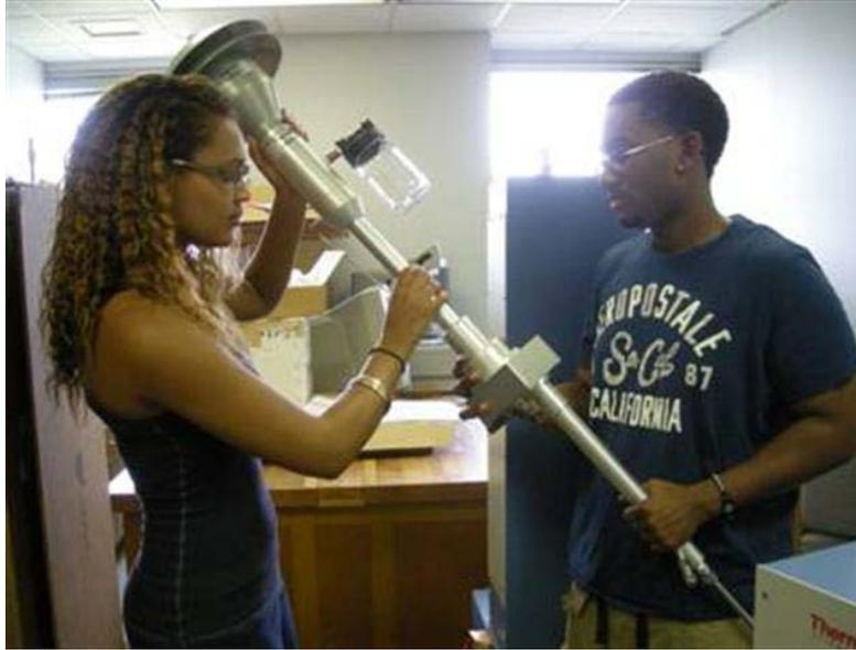
Figure 1. Students Avian Lain and LaMarr Hill installing the sample inlet tube into the section containing the virtual impactor and flow splitter.
