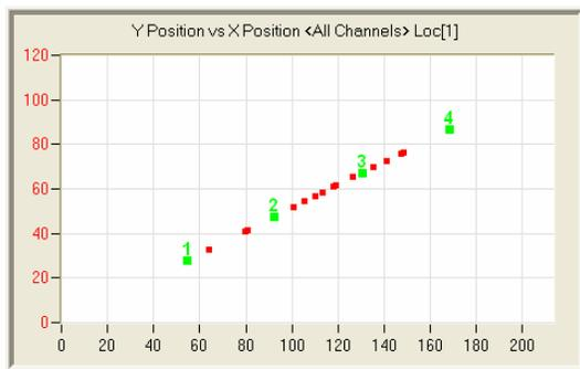
Fig. 8(a): AE Sensor locations on North Span of the cable
