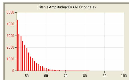
Fig 8(d): AE hits and their amplitudes
