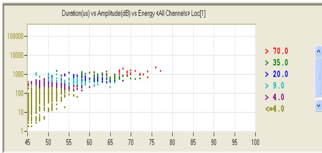
**Figure 11. Duration, amplitudes and energies of AE hits recorded by sensor 1 during an experiment in October, 2009**
