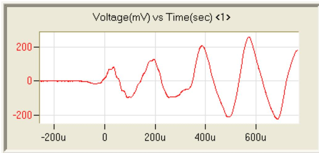
**Figure 5. An AE event representing pre-existing concrete crack rubbing recorded by sensor 1**
