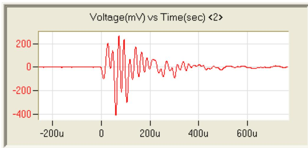
**Figure 6. An AE event representing pre-existing concrete crack rubbing followed by high energy counts of short duration representing crack formation/crack expansion recorded by sensor 2**
