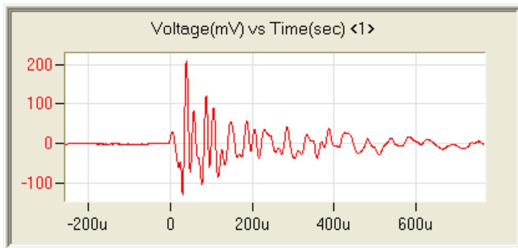
**Figure 8. An AE event representing initiation of a lower energy longer duration rubbing recorded by sensor 1**
