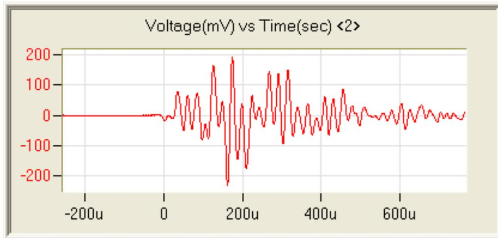
**Figure 7. An AE event representing crack formation followed by rubbing recorded by sensor 2**
